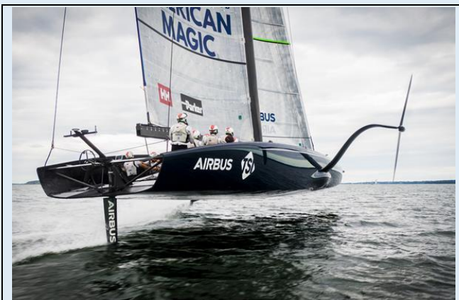
Defiant, the first of two AC75 foiling monohulls built by the New York Yacht Club's American Magic Syndicate.
