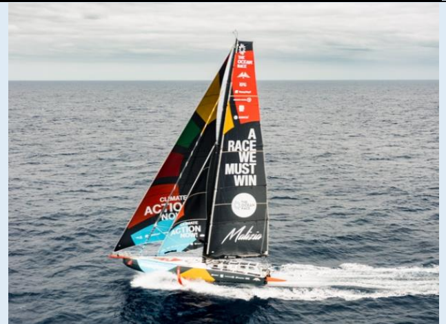
Team Malizia at speed. The orange tip of the port foil is visible along with one of the rudders, retracted for maximum speed.
